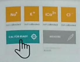
1 Initiate smart sensor calibration directly in main screen
