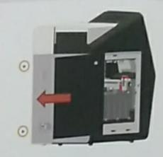
Remove left side panel to access valve V5
